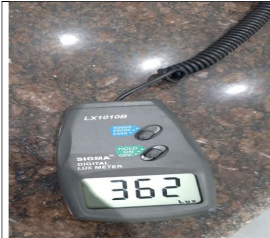
G1: Auditorium's LUX METER READINGS
